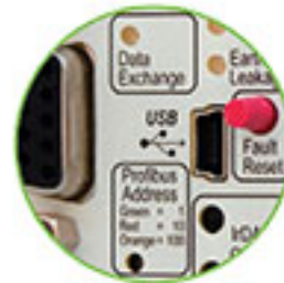
IRDA & USB Communication & Profibus address indication.
